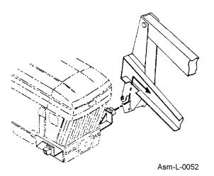
5. Clamp hinge assembly of upright around tube of midmount assembly. Install bolts, washers and nuts, and securely tighten.
